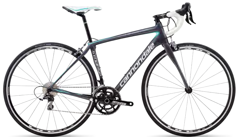
FRAMESET: Synapse Women's, BallisTec Carbon WHEELSET: Shimano RS01 CRANKSET: FSA Gossamer, BB30A, 50/34 COCKPIT: Cannondale C3 Women's GROUP: Shimano 105 / Tiagra COLORS: Charcoal Gray w/ Turquoise - Matte (01)
