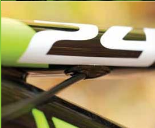
Internally Routed Cables
